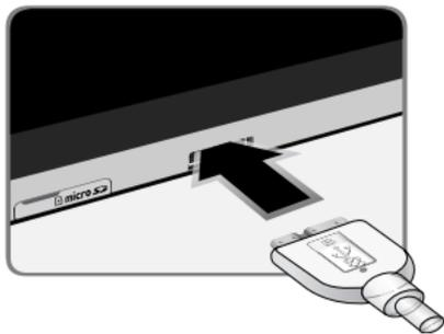
2. Insert the USB 3.0 cable into the Charging Head.
