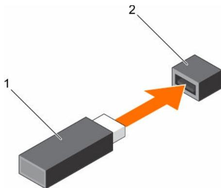
**Figure 48. Installing the internal USB key**
