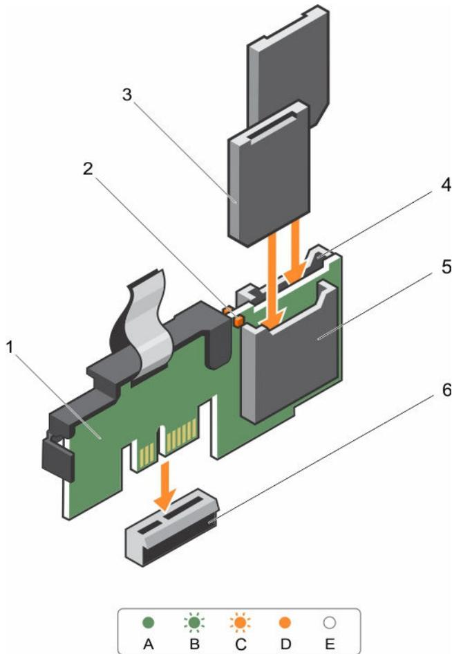
**Figure 58. Installing the optional internal dual SD module**
