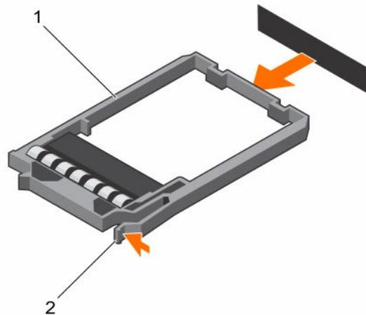
**Figure 31. Removing a 1.8-inch hard drive blank**
