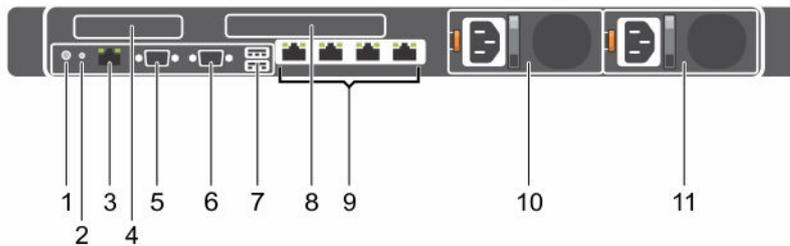
**Figure 6. Back panel features (two PCIe expansion cards)**
