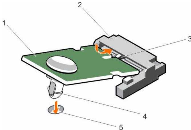
**Figure 99. Installing the TPM**
