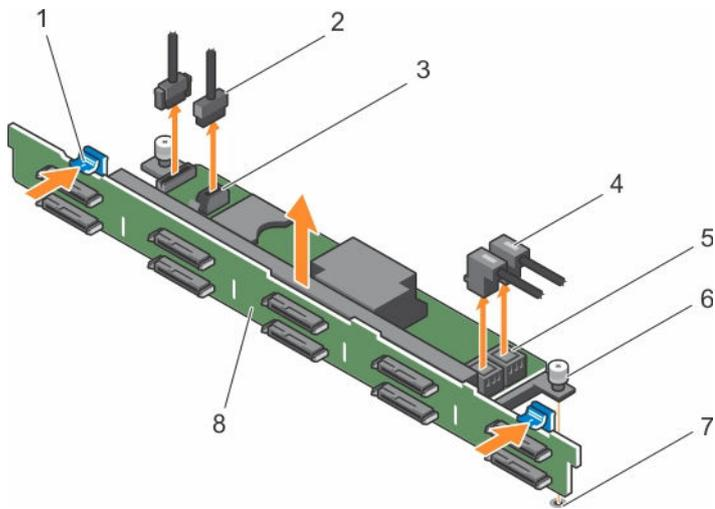
**Figure 82. Removing the 2.5-inch (x10) hard drive backplane**
